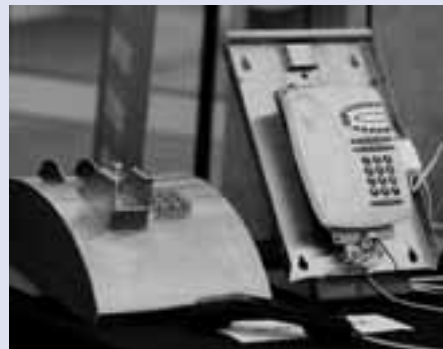
The robust community phone comprises a standard community phone placed within a weather-resistant steel casing
